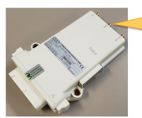
Both Versions of Controller (3 or 4 connector) are Interchangeable
